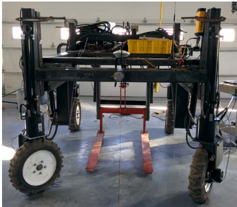
Fig 1. Bin-dog prototype with four-wheel-independent-steering
