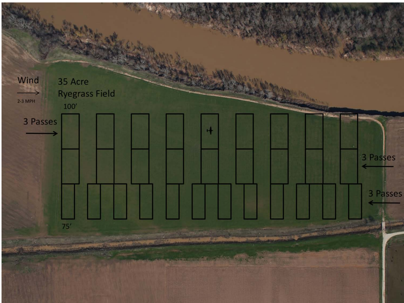
Figure 1. 35-acre ryegrass field with prescription application map overlay used for testing the system response of a variable rate aerial application system. The black boxes are 75' and 100' spray zones where 3 GPA of glyphosate solution were sprayed.
