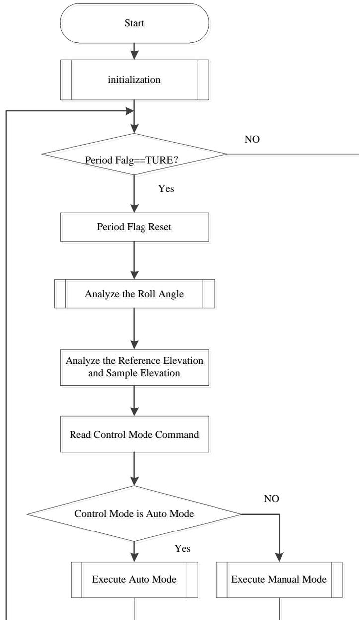
**Fig.7 Flow chart of monitor module**
