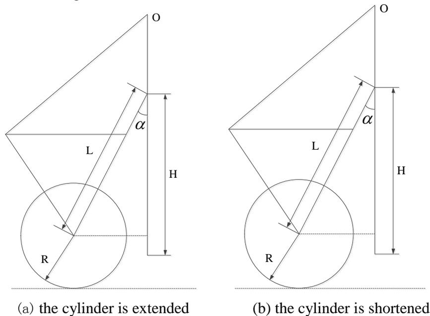
**Fig. 3 Blazer lifting mechanism when the cylinder is extended**
