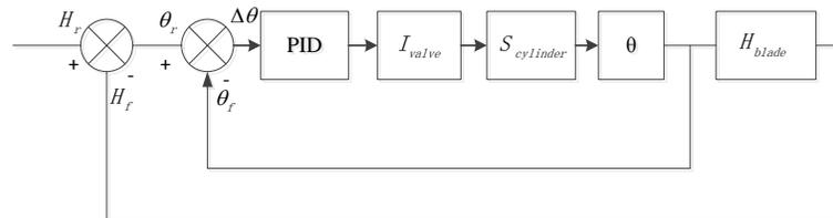
**Fig. 5 Control system of blade lifting mechanism**
