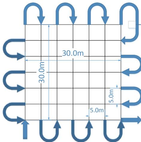
**Fig.8 Routing of land measurement**
