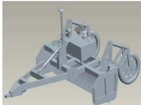
**Fig. 1 Mechanical structure of GNSS land leveling equipment**
