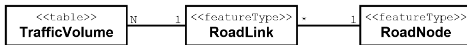
Fig 7. Open Transport Map data model geometrical elements created as a consensus of the FOODIE, OTN and SDI4Apps.
