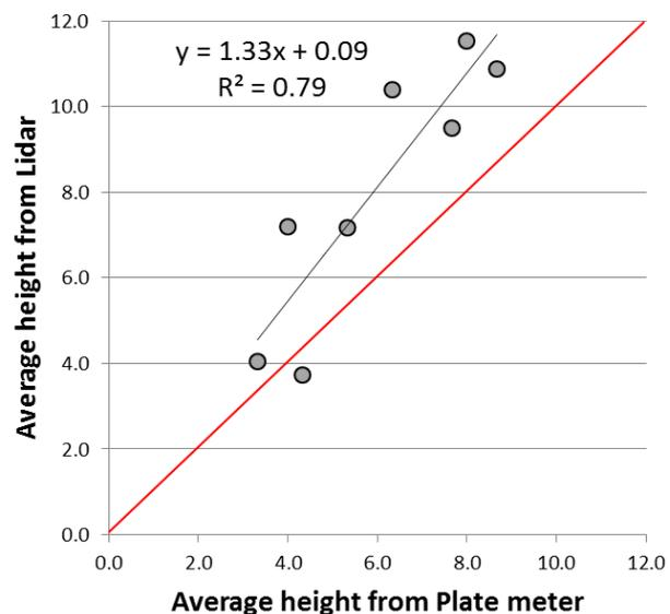
Figure 2. Relationship between the average height from a plate meter and the average height from the LidarLite sensor. Red line depicts the 1:1 line.
