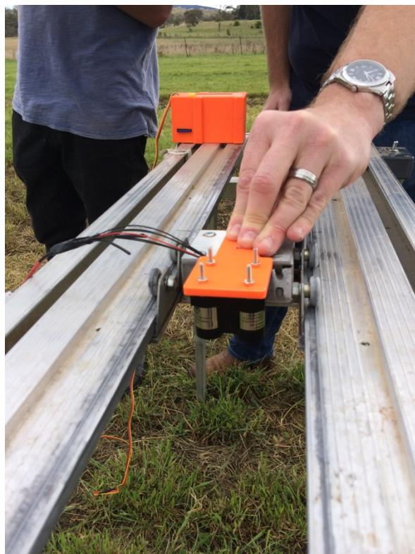
Figure 1. The LidarLite™ sensor mounted on sampling table with data logger.
