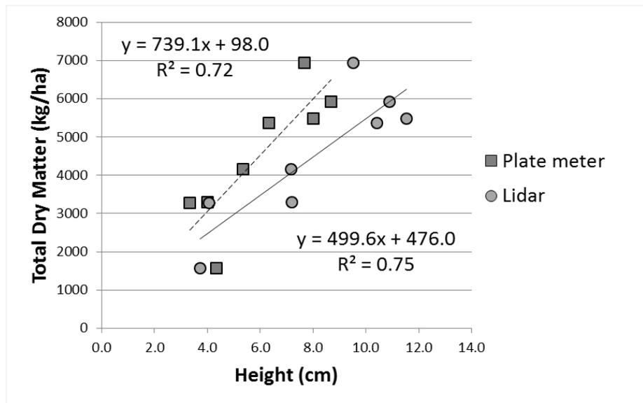
Figure 3 Comparison between the Plate meter and Lidar in terms of the correlation to Total Dry Matter (kg/ha). Both sensors show a similar calibration accuracy.
