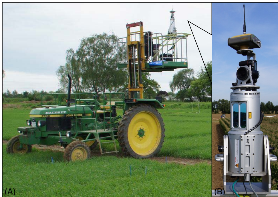
Fig. 2. Instrumental set-up: (A) Tractor with hydraulic platform; (B) Terrestrial laser scanner Riegl LMS-Z420i with digital camera Nikon D200 and RTK-DGPS receiver on top.
