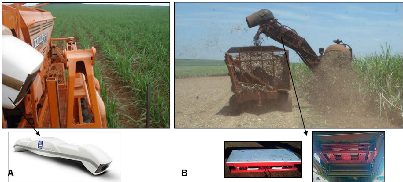
Fig 1. Data collection by crop canopy sensor scanning (A) at early season and harvest with yield monitor (B)
