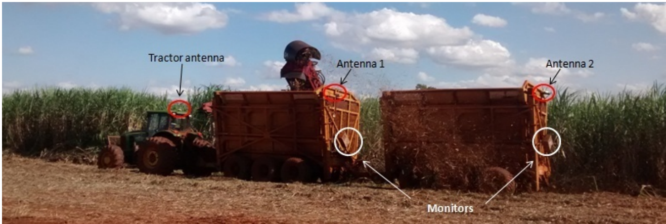
Figure 1 - Schematic representation of the arrangement of GNSS antennas in the set
