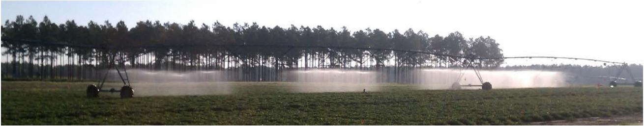
Fig 1. VRI-enabled pivot at UGA's Stripling Irrigation Research Park being used to vary irrigation application rates over research plots.
