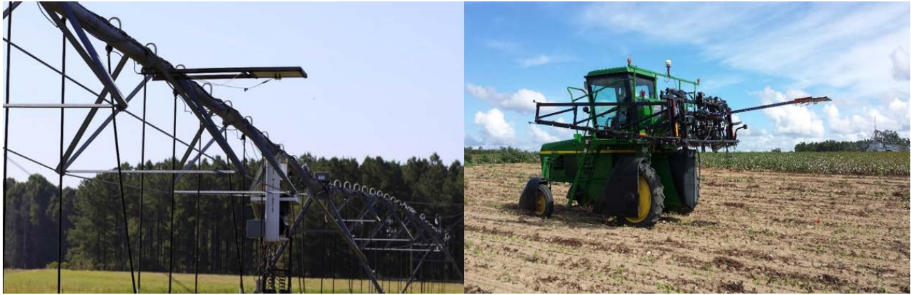
Figure 1. GPS antennas mounted on lateral VRI (left) and on a high-boy sprayer (right) during 2013 and 2014, respectively.
