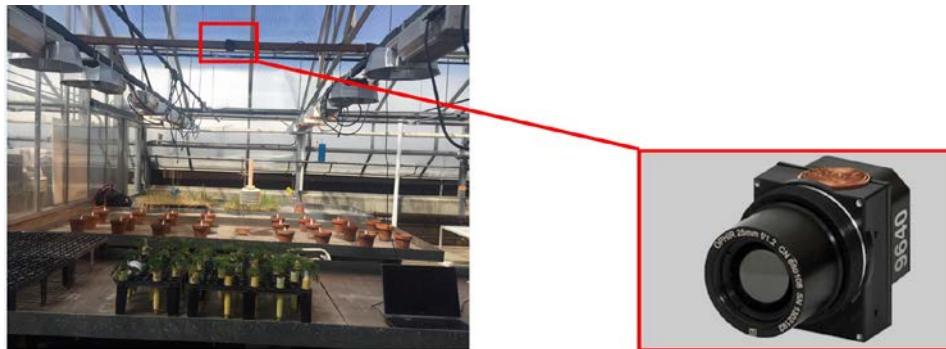
Figure-1. Thermal images in NDSU greenhouse, with a close-up of the thermal camera.
