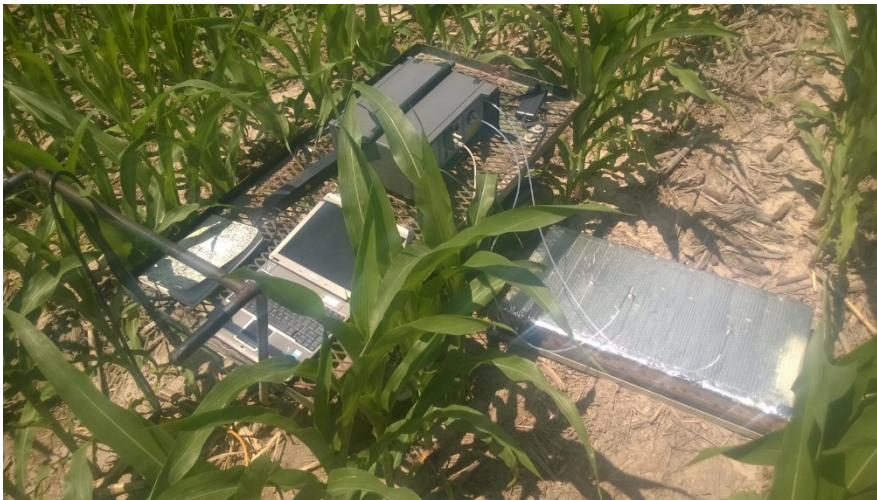
Figure 3. Nitrous oxide concentration measurements are made for 14 minutes under a chamber that spans from one row to the next using a photoacoustic spectrometer. The measurement area is uncovered except during flux measurements.
