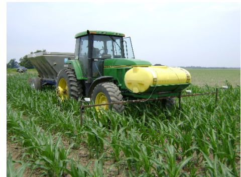
Figure 1. Crop Circle ACS-210 sensors on dry fertilizer spreader, variably applying N based on crop color.
