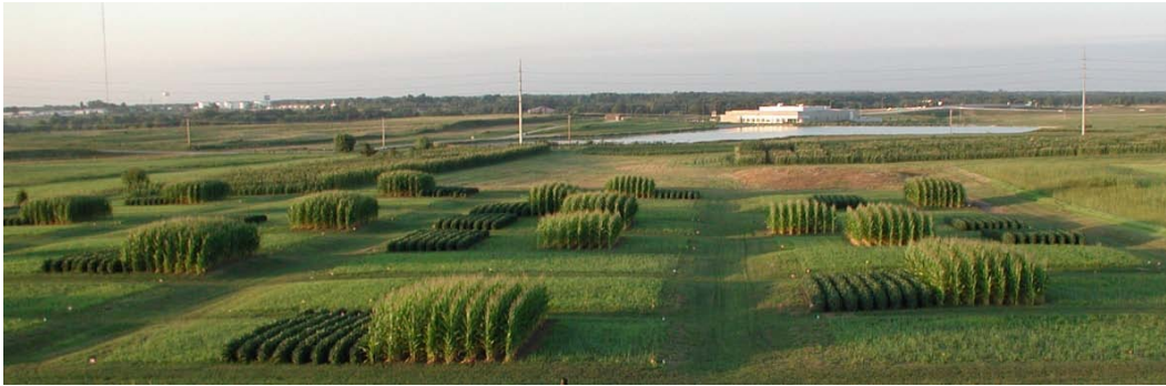
Photo 1. The layout of the 32 SPARC plots at the University of Missouri South Farm showing corn, soybean, and switchgrass growing on blocks of varying topsoil depth.
