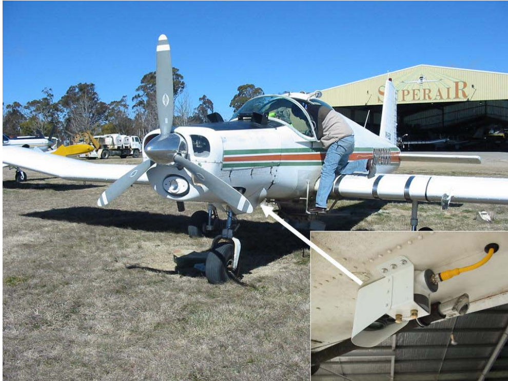
Figure 1. Photograph of the Fletcher FU24954 (VH-EQC) crop-dusting aircraft and the CropCircle mount (inset). The sensor was positioned in a nadir-view configuration with the long-axis of the LED array at right angles to the flight direction.
