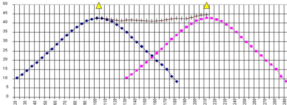
**Figure 4. Illuminations in lux obtained for two power-leds separated by 110 cm.**
