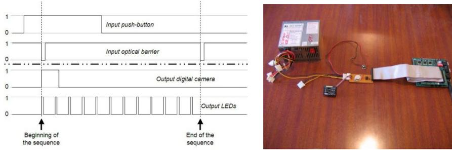
**Figure 2. The whole stroboscopic command and functioning sequence.**
