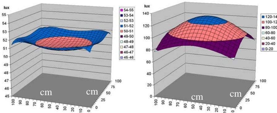
**Figure 5. Best illumination of the field of view with four power-leds located on a square (left) or six power-leds located on a hexagon (right).**
