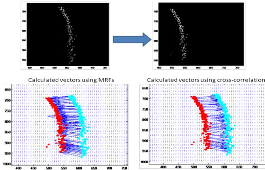
**Figure 9. Velocity vector fields obtained with MRFs (bottom left) and cross-correlation (bottom right) techniques, between two successive throws (up right and left).**
