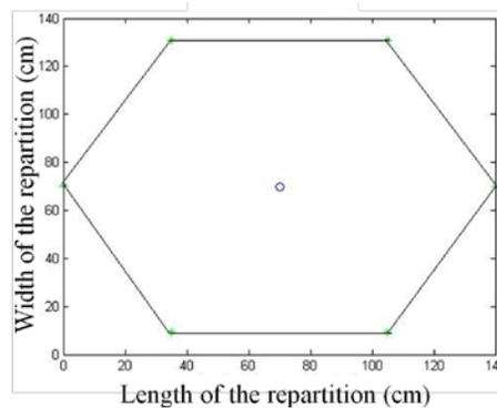
**Figure 6. New hexagonal arrangement with eight power-leds at each location.**
