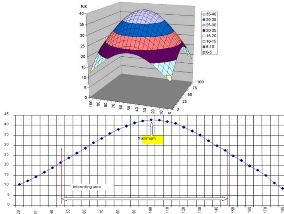
**Figure 3. Illumination in Lux of one single 3W power-led located at the centre of the field of view.**
