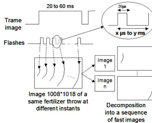
**Figure 1. Principle of the high-speed imaging device and example of typical multiexposure image obtained.**
