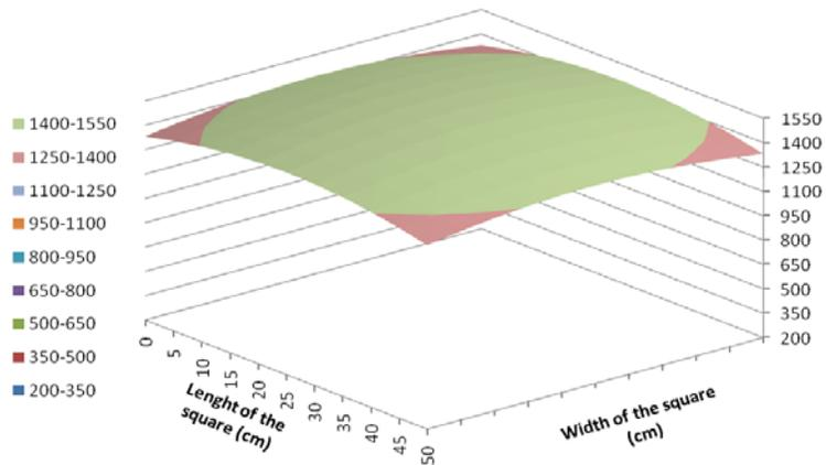
**Figure 8. Illumination (in lux) for 72 3W power-leds uniformly arranged on a hexagon inscribed in a circle with a radius of 25 cm.**
