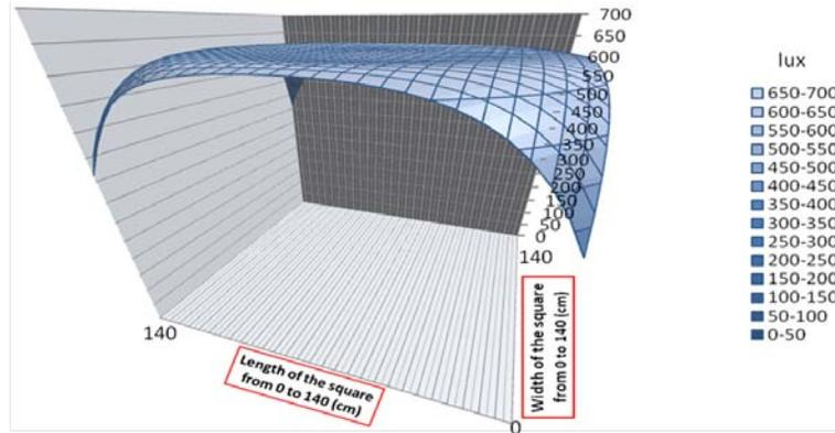
**Figure 7. Illumination (in lux) for 48 3W power-leds uniformly arranged on a hexagon inscribed in a circle with a radius of 70 cm.**
