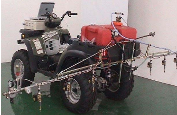
Figure 2: Automatic Sprayer Installed with Web Camera and Communication Devices.
