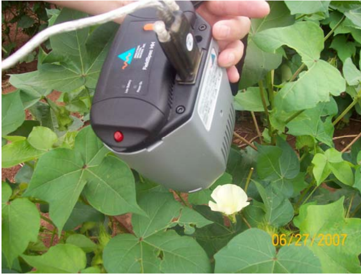
Figure 5. FieldSpec radiometer was used to measure crop conditions
