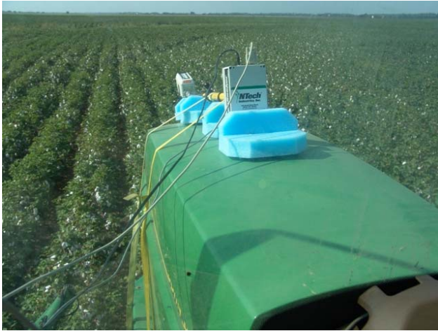
Figure 4. GreenSeeker Model 505 Handheld Optical Sensor Mounted on John Deere 4710 Variable-Rate Sprayer with 90' Swath for Ground-Mapping NDVI in Cotton Field.
