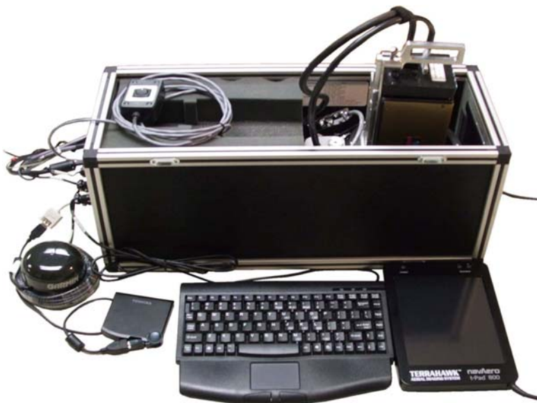
Figure 2. Complete camera control system assemble.
