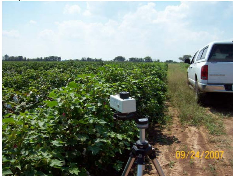
Figure 3. An irradiance radiometer was used to record Sun's irradiance in the field.
