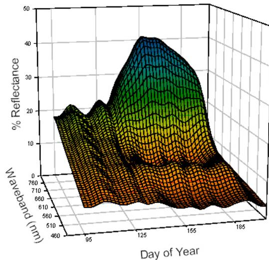
Figure 3. Reflectance over canola during the 2007 growing season obtained with a CropScan eight-band radiometer.
