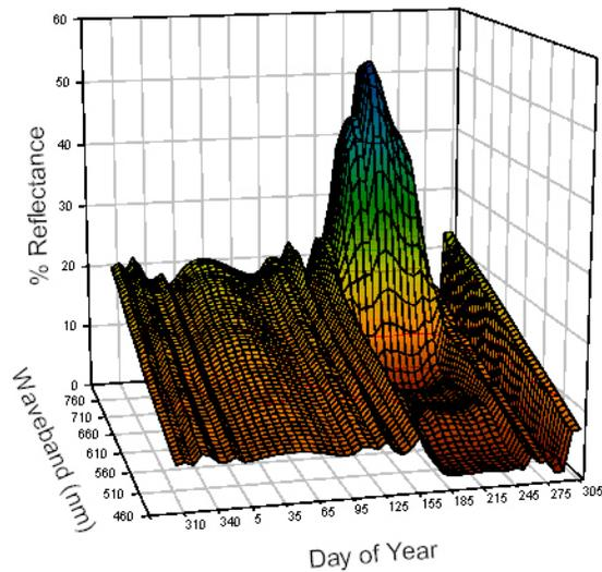
Figure 1. Reflectance over corn obtained throughout the year with a CropScan eight-band radiometer over a spring strip tillage system.
