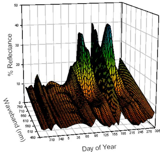
Figure 2. Reflectance over wheat (until DOY 180) and soybean (DOY 180 and greater) obtained throughout the 2006- 2007 year with a CropScan eight-band radiometer.
