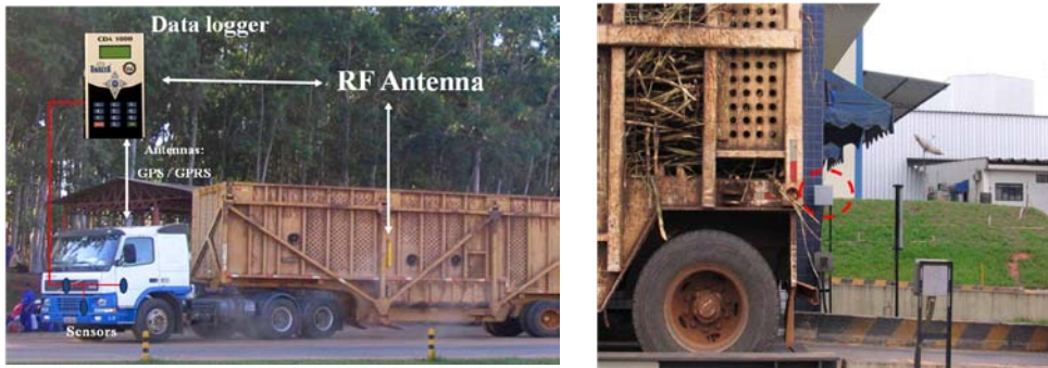
Fig. 4. Reception radio installed on weighing site of sugar cane mill
