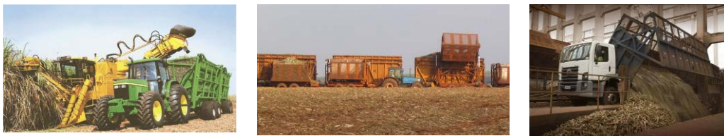
Fig. 1. CCT operation: harvesting (cutting), hauling (caring) and transportation of sugar cane from field to the mill.
