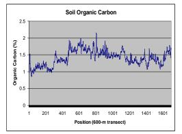
reflectance measurements and expressed as organic carbon content. A sample of the data shows the sensor (green and NIR wavebands) is responsive to soil brightness. The sensor and coulter apparatus worked very well to cut through residues. Soil brightness measurements were taken at ~10 cm depth.
