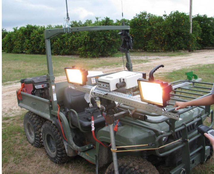
Fig. 2. Data capturing system including hyperspectral radiometer and artificial illumination
