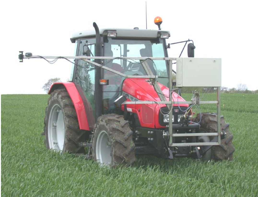
Fig. 1. MobilLas sensor mounted at the front of a farm tractor. PC, power supplies etc. are housed in the box placed at the centre of the sensor frame. System monitor and keyboard placed in the tractor cab. GPS receiver and ASC-210 radiometer are mounted at the end of the long boom. The laser range finder is mounted on the short boom at an off nadir angle of 50 deg.
