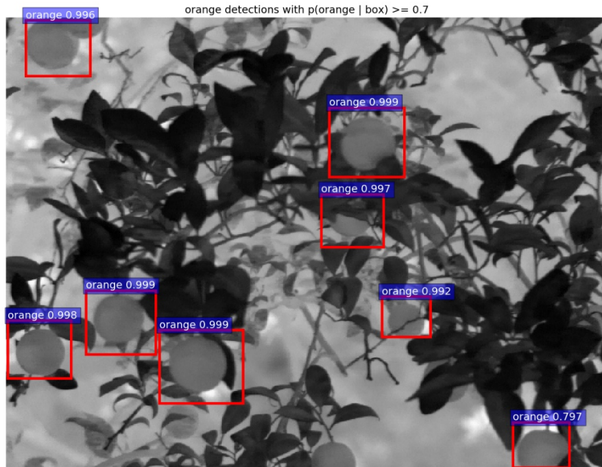
Fig. 4. Example thermal images of citrus canopies after spray. The detected fruit was labeled with red rectangles and confidence values
