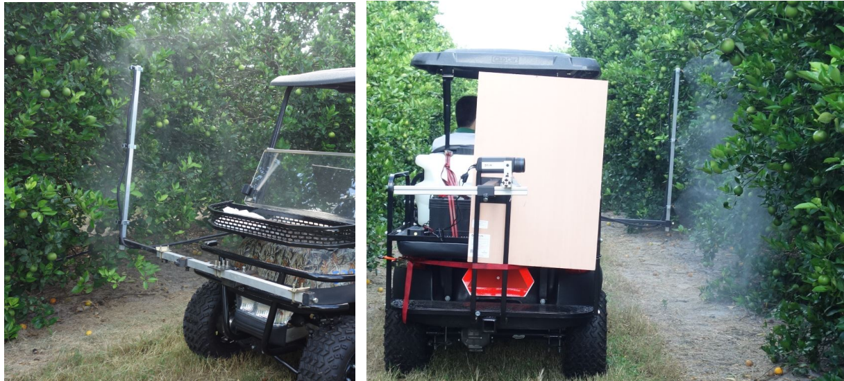
Fig. 1. The imaging system. Left: the metal bars and three nozzles mounted vertically on the bar. Right: A view from the back of the entire imaging system
