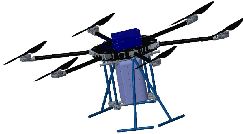
Fig.3.1. CAD Assembly of complete prototype with 20-liter payload.
