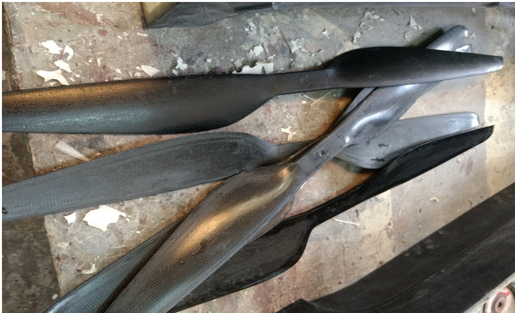
Fig 4.2. The indigenized carbon fiber propellers developed at Reinforced Plastic Industry.
