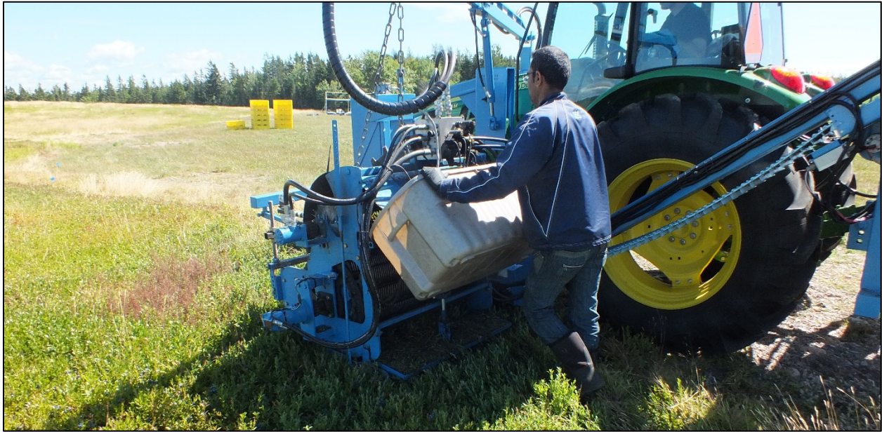
Fig. 3 Manual collection of debris removed by cleaning brush from picker teeth and flung clear of harvester head.
