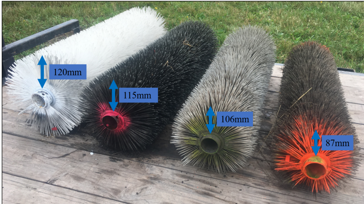
Fig. 2 Debris cleaning brushes with different wear levels used for field experimentation.
