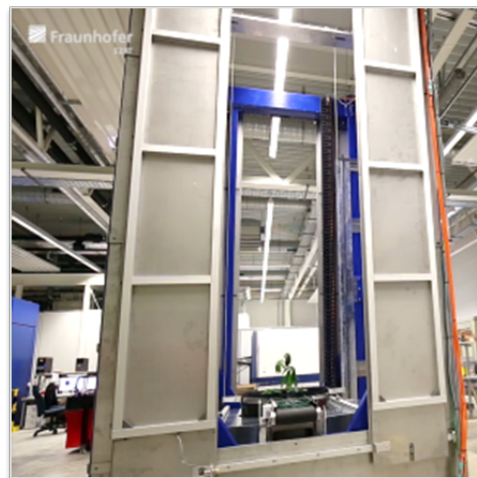
Fig. 11: Measurement system for automated root analysis
