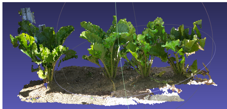
Fig 3: Color 3D data generated from 3-camera setup
