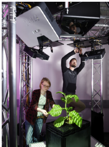
Fig. 8: Using structured light projection to measure tobacco plants
