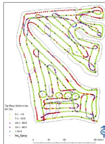
Fig. 1. Tip flow rate uniformity (%) for spray application with travel direction for Field A.
