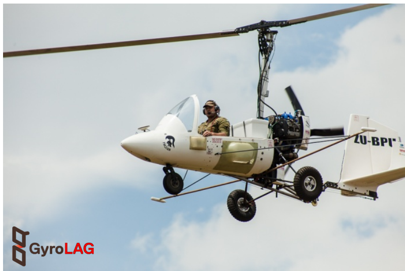
Fig. 3 GyroLAG highly modified South African gyroplane Trojan equipped also with geophysical instruments.
