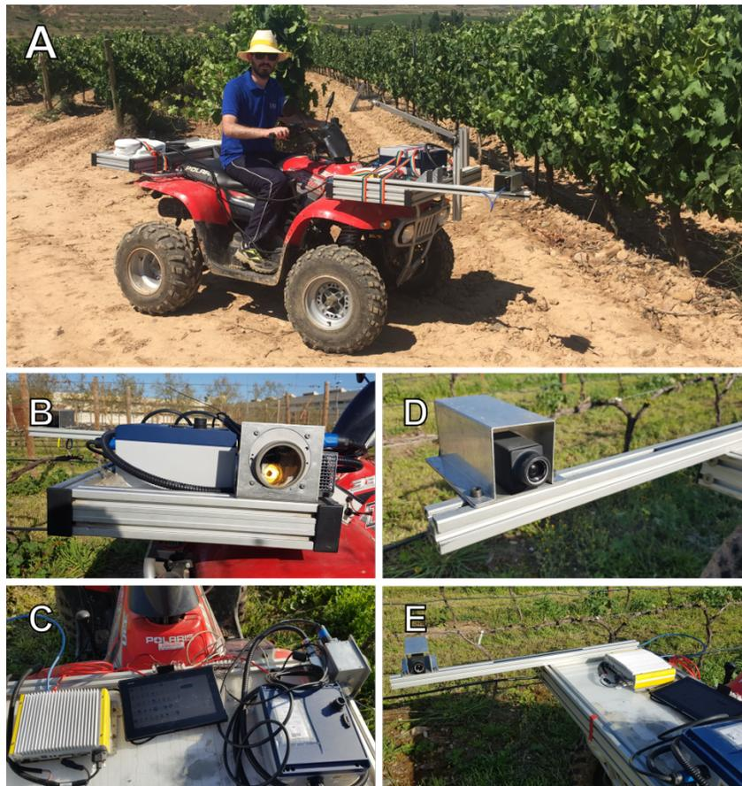
**Fig 1. (A) General display of the all-terrain vehicle mounting thermal imaging and NIR sensing technologies for assessing vineyard water status. (B) Detail of the NIR head sensor. (C) Industrial computer, control tablet and NIR processing unit and head sensor. (D) Detail of the thermal camera. (E) Industrial computer and control tablet for the thermal camera.**
