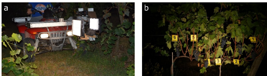
Fig 1. (a) On-the-go image acquisition with the modified ATV; (b) Image acquired using the artificial illumination system
