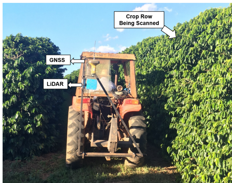
Figure 3. Tractor mounted structure for MTLs field data collection for coffee
