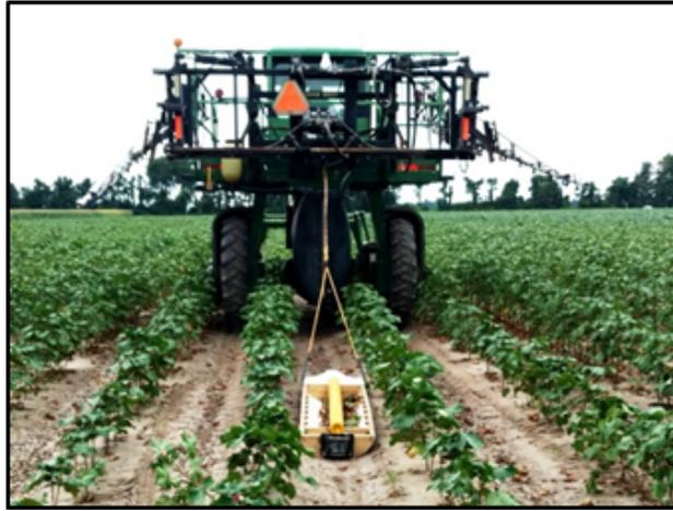
Fig. 4. DUALEM 1HS instrument collecting within-season  $EC_a$  data in cotton field.
