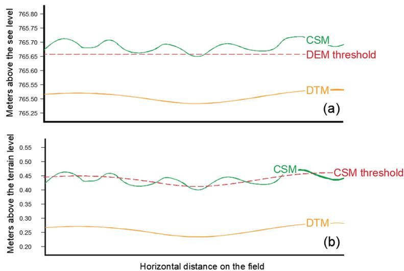
Figure 5. Effect of using directly the DEM (a) to create the plant height threshold, compared with using CSM (b).
