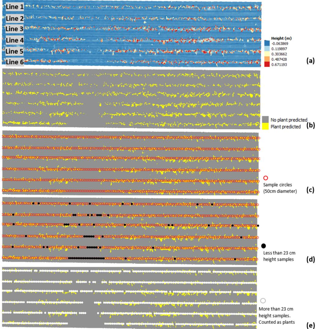
Figure 3. Resulting images from the main steps of the process: (a) DSM, (b) planted and non-planted areas binary image, (c) circular sample zones, (d) samples not counted as plants and (e) samples counted.
