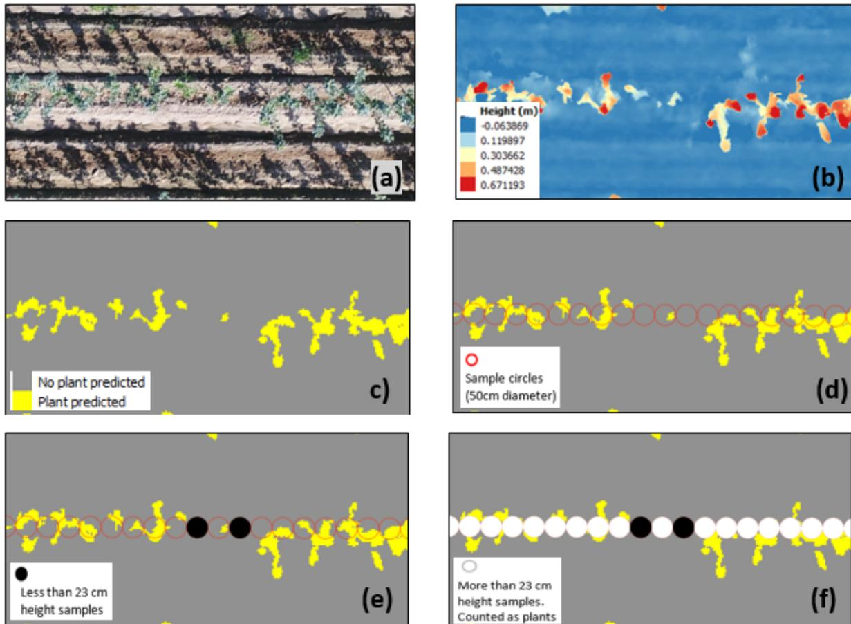
Figure 6. Example of processing steps from the original image (a) until the identification of plants (f), passing through CSM (b), binary image (c), sample regions (d) and thresholding (e).
