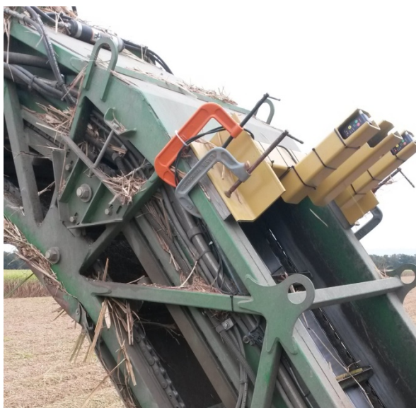
Figure 1. Experimental yield monitor sensor bar mounted on harvester conveyor.
