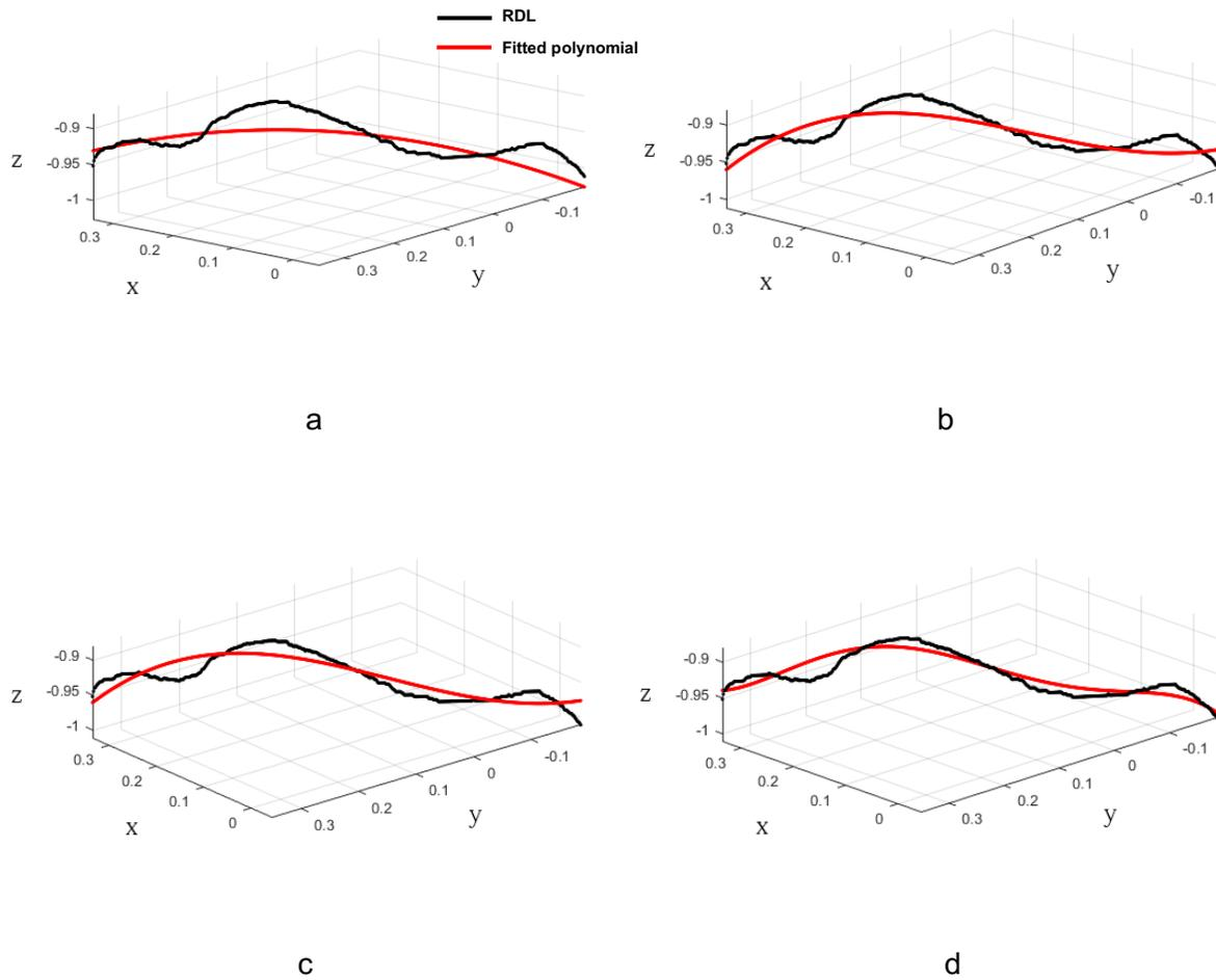
Fig. 2 Polynomials fitted on RDL at  $\theta = 55^\circ$  from a cow with BCS 3.5; a) order of 2, b) order of 3, c) order of 4, d) order of 5. The normalized area bounded to these two lines were used in the ripple factor as the extracted feature
