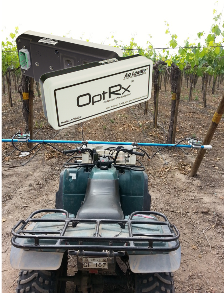
Figure 1. Active sensors OptRx mounted on ATV.
