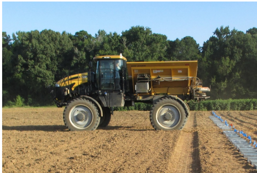
Figure 1. Image of standard pan collection testing. Fertilizers are applied over the pans, then mass is quantified and an assessment of spread uniformity is generated.
