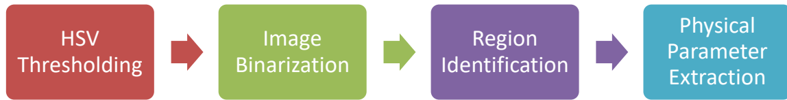
Figure 3. Image processing steps to acquiring needed information for applied mass calculations.
