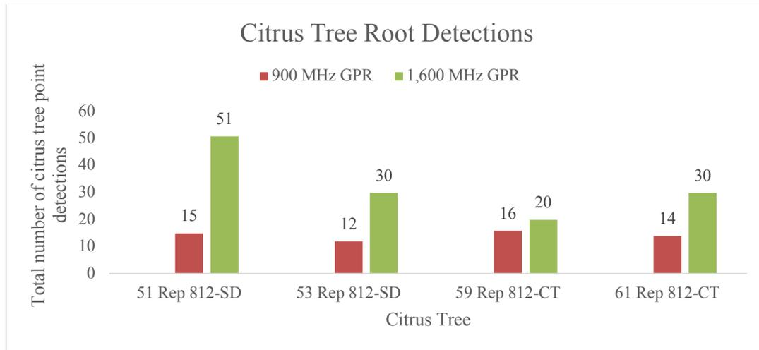
**Fig. 5.** Citrus tree root points detection by the: (i) 900 MHz GPR, and (ii) 1,600 MHz GPR.
