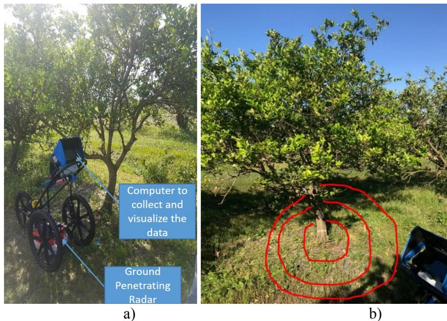
**Fig. 1.** a) A ground penetrating radar (GPR) mounted to a scanning cart; b) 360-degree peripheral scans around the tree trunk to detect tree roots.
