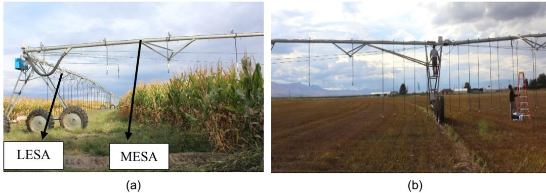
Fig. 1. LESA and MESA installed in the study area (a) Corn field (b) spearmint field. The emitters of LESA, as seen, are closer to the ground than MESA. Also, the outlet spacing of emitters in LESA is less by 3-6 m (10-20 ft).
