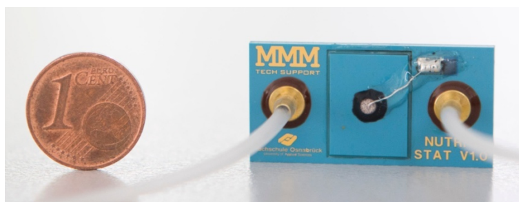
Figure 5: NUTRI-STAT ISFET sensor module; dimensions of the ISFET sensor module with plug-in socket (width, depth, height): 33 x 17 x 10 mm, (Image sources: University of Applied Sciences Osnabrueck)
