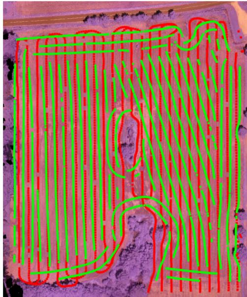
Fig. 2. Registered geo-referenced soil and yield data plotted on an orthomosaic image. The red line indicates the route of ECa soil survey and the green line indicates the route of harvesting
