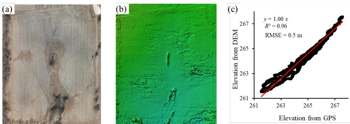
Fig. 3. Elevation measured with imaging method. (a) RGB orthomosaic image of test field taken prior to planting. (b) DEM map generated based on images and (c) fitness between elevations measured by imaging method and a RTK GPS system.
