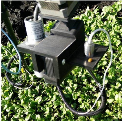
Fig. 1. Picture illustrating the 3D-printed sensor holder
