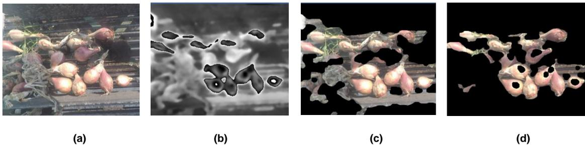
Fig. 7. Segmentation results. (a) Original conveyor image and results (b, c, d) of the image processing and segmentation algorithm. (b) is the red color intensity image, (c) is the image segmented using Otsu’s method (d) is the segmentation performed using the manually selected hue and saturation thresholds.
