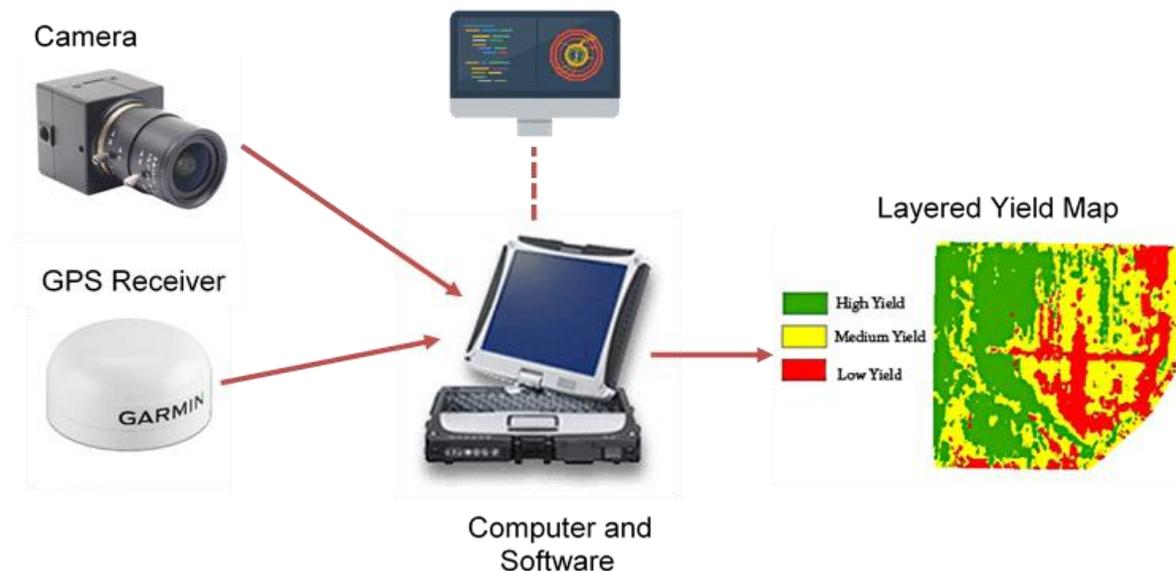
Fig. 3. Diagram of the machine vision yield mapping system. The camera records continuous video of the crops being collected by the harvester. Each frame is coupled with a location tag given by the GPS receiver. The data is analyzed using a computer vision software and exports a yield map showing the size distribution of the crops per unit area.
