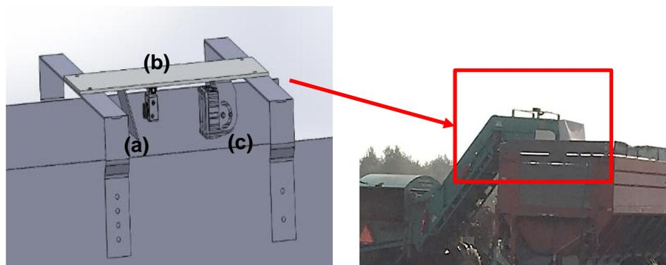
Fig. 2. Model of the machine vision camera bracket (left), (a) is a metal piece used to deflect incoming onions from the camera (b), and (c) is the external light source. Right image is the setup positioned on the farm harvester.
