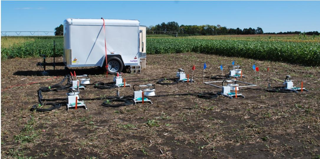
**Fig. 1.** Setup and configuration of Picarro Spectrometer and LI-COR chamber units at the Aurora Research Farm, Fall 2017. Picarro and LI-COR analysis equipment was housed in white weatherproof trailer in background.
