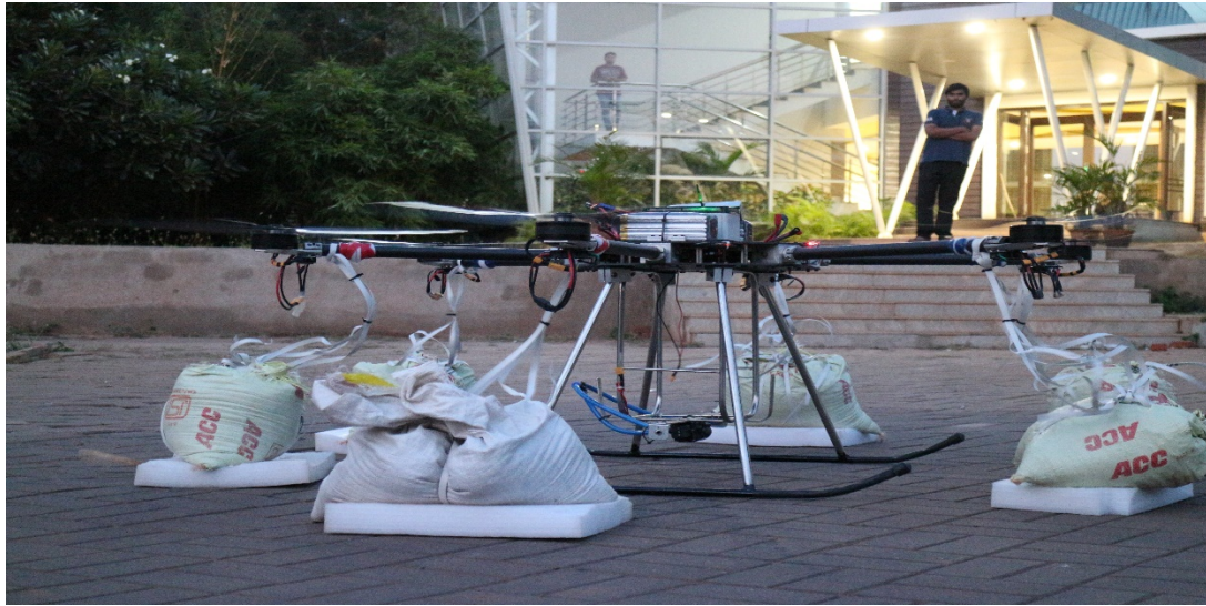
Fig 4.3. The sand weights suspended to UAV arms for takeoff calibration.
