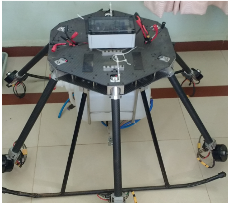
Fig 3.5. Folded prototype for storage and transportation.
