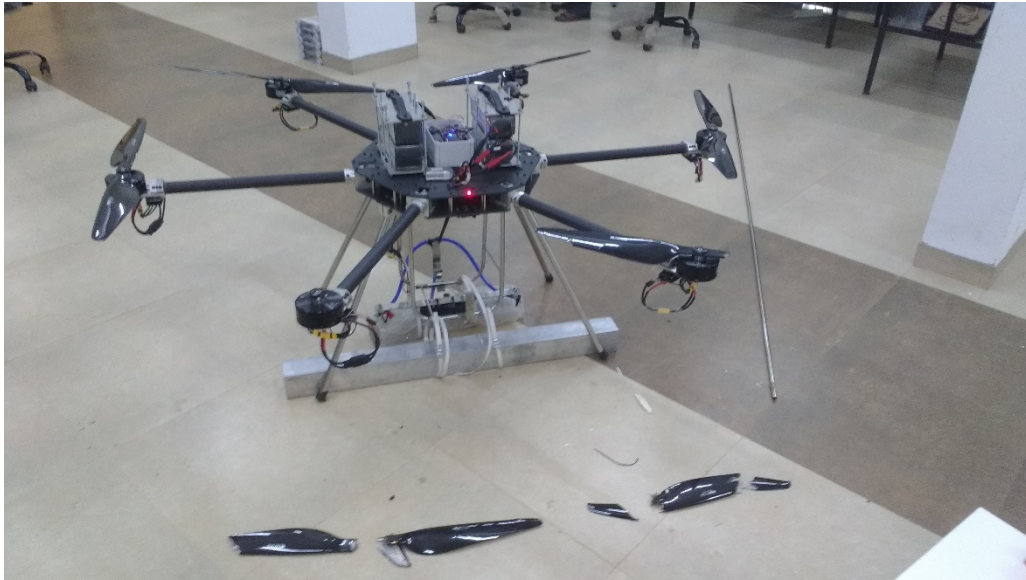
Fig 4.1. Crash site of prototype unmanned aerial sprayer, with broken propellers.
