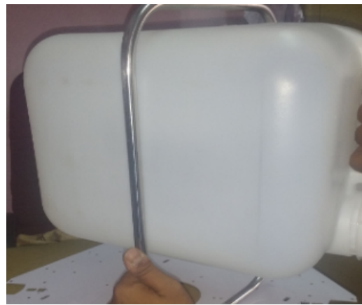
Fig. 3.2. (b) The cage assembly for HDPE Payload.
