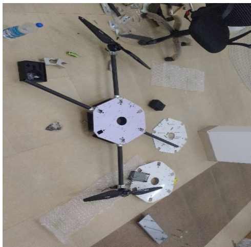
Fig 3.3. In house Assembly of dummy prototype for mount verification.
