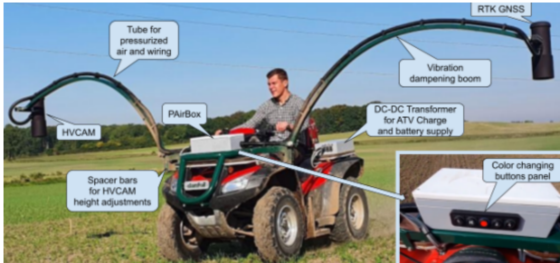
Fig 1 – ATV mounted with the RWM dual camera system, and additional components
