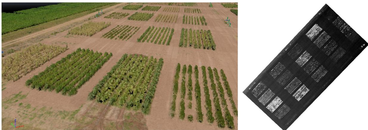
Fig. 2. Point cloud (left) and digital surface model (right) for 16 test plots based on images taken at 60 m on 8 August 2019. On the right map, light gray color represents high elevation, whereas dark gray color depicts low elevation.
