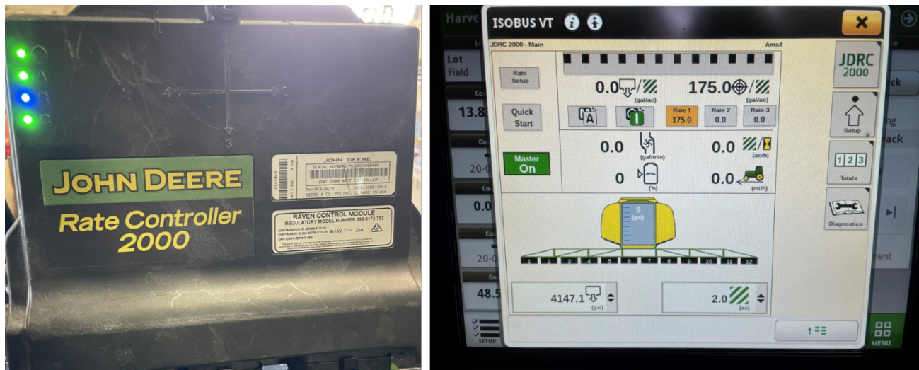
Figure 3: John Deere's RC2000 Universal rate controller (left) and 4640 display (right) showing the interface for the 12-nozzle sectional control for the applicator (right)
