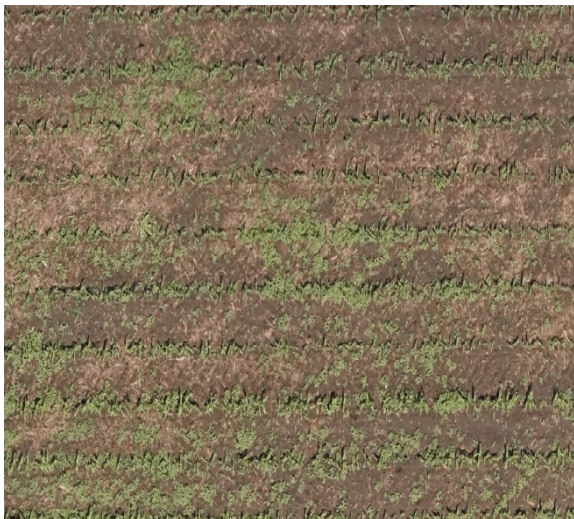
Fig 4: UAV image of corn rows with resolution of 1 cm. Besides the crop rows, weeds can be identified in the top left, center, and bottom right.
